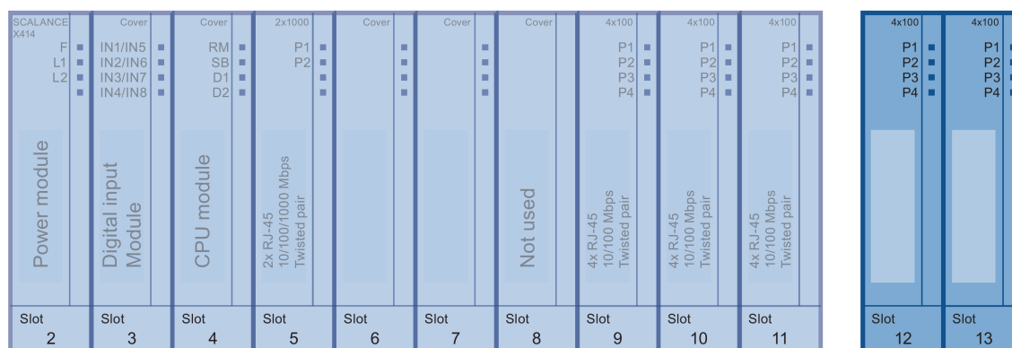
Figure 3-27 Basic device with twisted pair extender module
