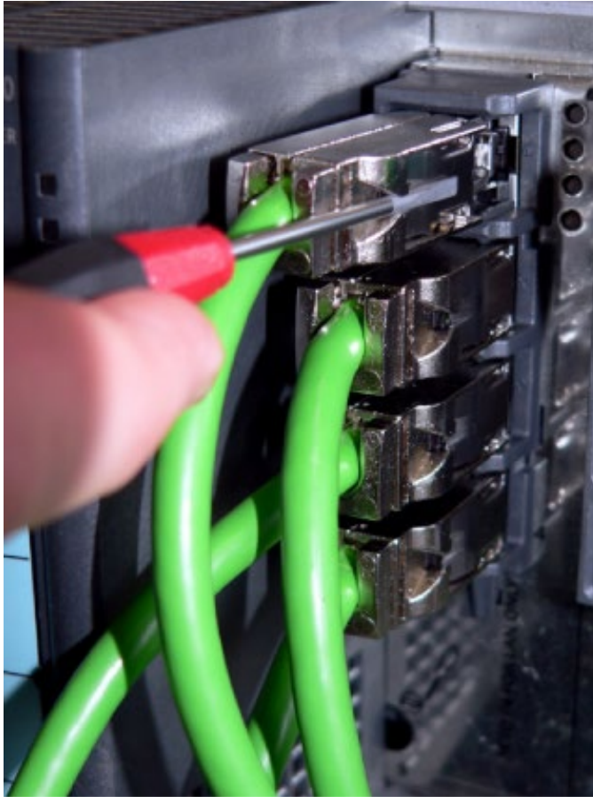
Figure 5-9 Unlocking the FastConnect RJ-45 plug
