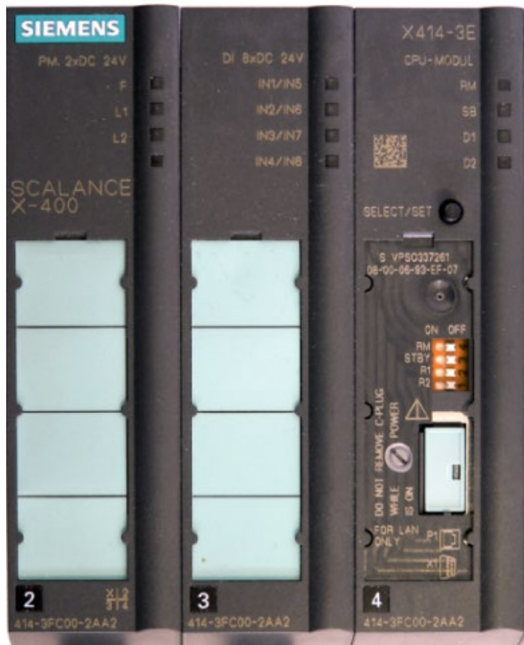
Figure 6-2 Power module, digital inputs and CPU module with operator controls on the SCALANCE X414-3E
