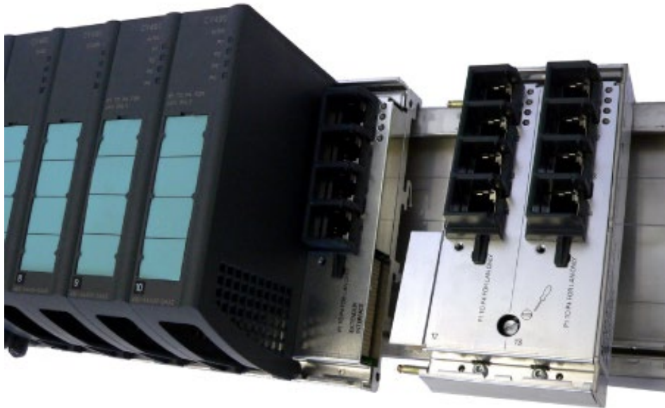
Figure 4-6 Installing the twisted pair extender on the S7-300 standard rail
