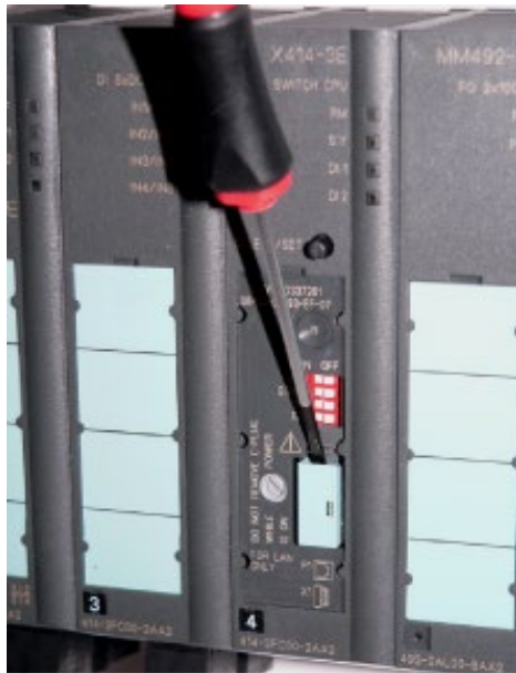
Figure 6-13 Removing the C-PLUG from the SCALANCE X414-3E
