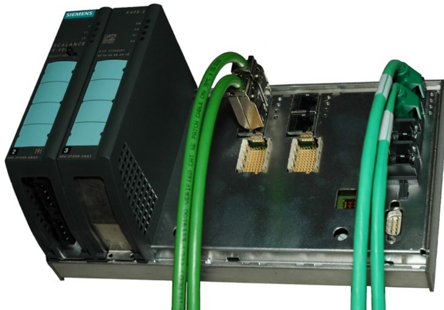
Figure 3-24 Basic device with gigabit cable and Fast Ethernet twisted-pair cable
