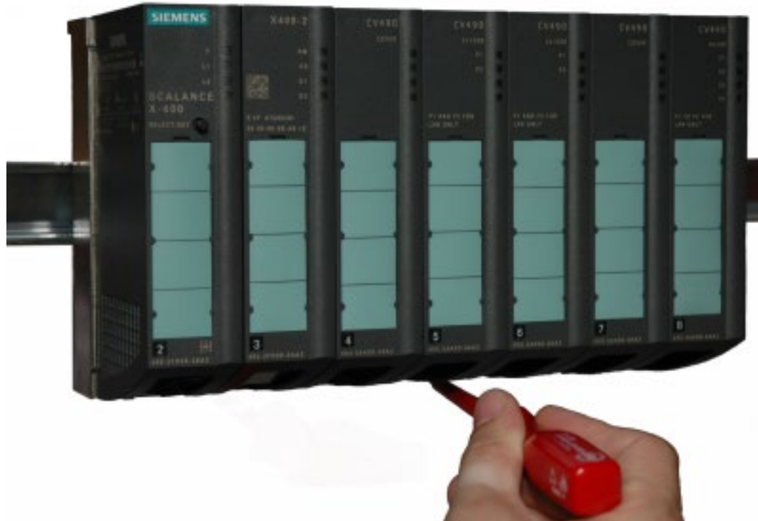
Figure 4-4 Removing the SCALANCE X408-2 from a 35 mm DIN rail
