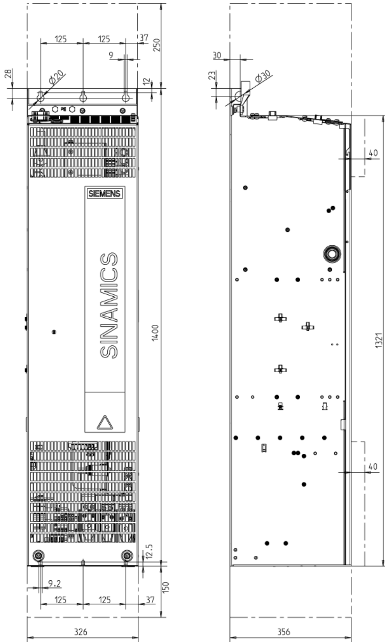
Figure 5-6 Dimension drawing Motor Module, frame size FX. Front view, side view
