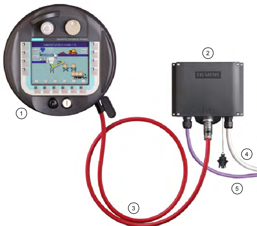
Figure 1-2 Mobile Panel 170 – Design
