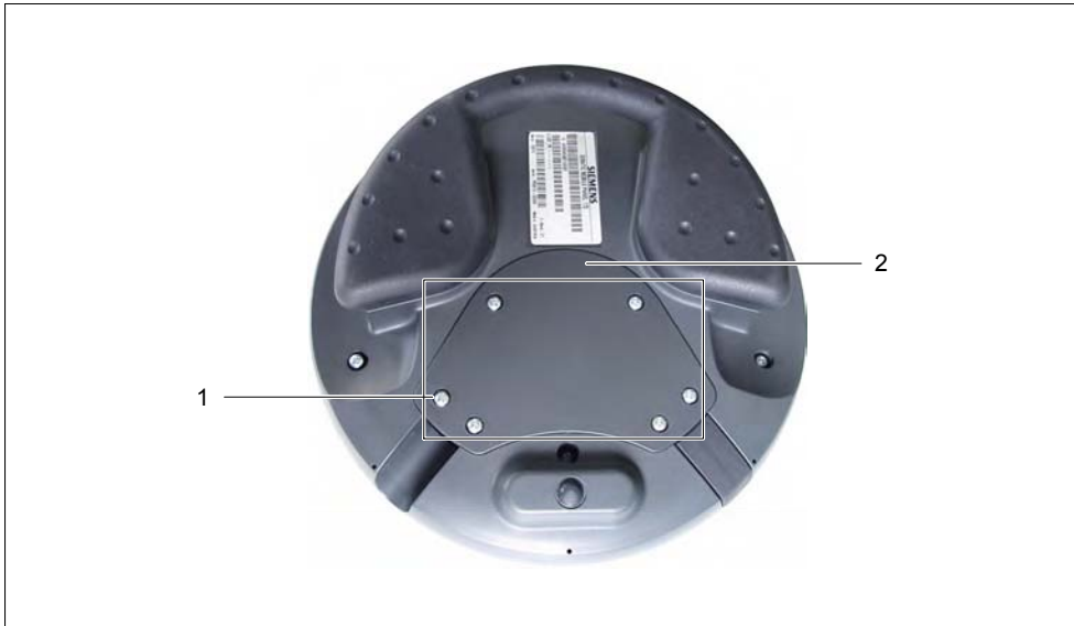
Figure 4-1 Opening the terminal compartment
