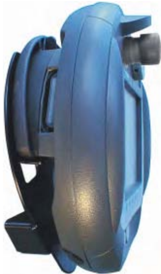
Figure 9-6 Mobile Panel 170 in the wall holder
