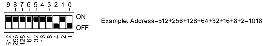
Figure 3-1 Example for setting the address switch (DIP switch)
