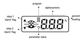
The SITRANS CU 02 normally displays the input signal level (Vsens) from the SITRANS sensor in volts, or in percentage of the programmed span (P3-P2). The selection is made while viewing Vsens.
