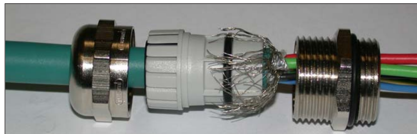
Fig. 2-29 Example: M20 gland with all of the individual parts
