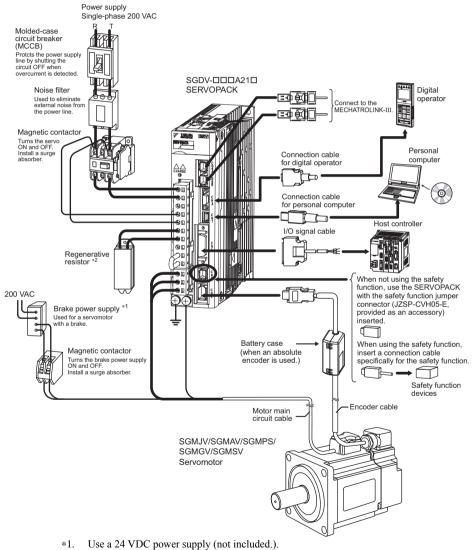
Before connecting an external regenerative resistor to the SERVOPACK, refer to 3.4 Connecting Regenerative Resistors. Wiring and Connection
