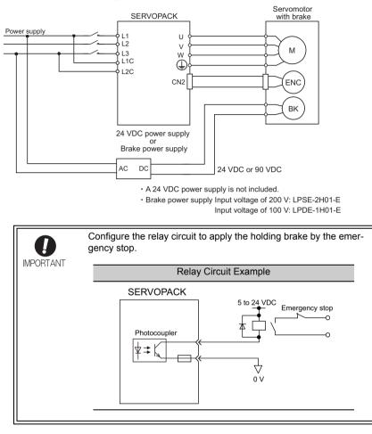
An example of the circuit wiring
