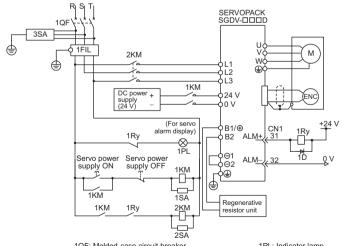
1QF: Molded-case circuit breaker 1FIL: Noise filter
