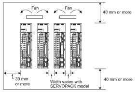
Leave sufficient space on each side and at the top and the bottom of each SERVO-PACK. The width on each side varies in accordance with the models of the SERVO-PACKS used.
