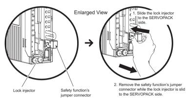
Note: The safety function's jumper connector may be damaged if removed while the lock is still on.
