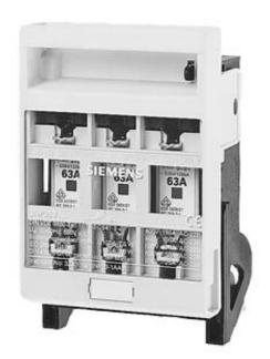
FUSE-SWITCH-DISCONNECTOR I = 100/160A, U = 500/400V TYPE OF CONDUCTOR CONNECTION: BOX TERMINAL FUSE SIZE NH00 (21MM WIDE)
