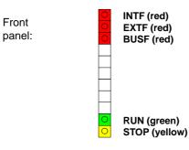
The different combinations of the five LEDs on the front panel indicate the status of the CP:
