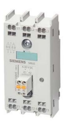
SOLID STATE RELAY 3-PHASE 3RF2 30 A 40 DEG. C 48-600 V / 4-30 V DC 2PH.-CONTROLLED SPRING-TYPE TERMINALS BLOCKING VOLTAGE 1200 V
