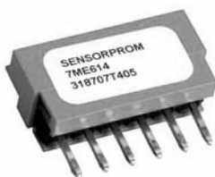
Figure 3-3 SENSORPROM memory unit
