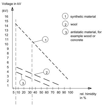
Figure B-1 Electrostatic voltages on an operator
