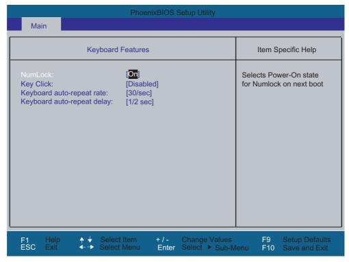
Figure 14-7 "Keyboard Features" submenu (Example)
