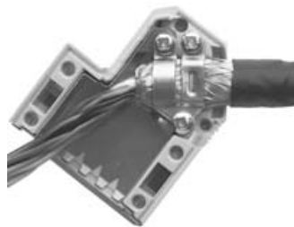
Figure 159: Connect the shield in the sub D connector
