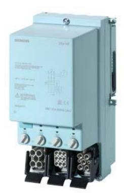
ET 200PRO RSE HF REVERSING STARTER HIGH FEATURE MECH. SWITCHING; ELECTRO. UE PROTECTION; 3PH 400 V/5.5KW; 1.50A...12.00 WITHOUT BRAKE CONTACT 4DI 24 V DC; HAN Q4/2 -HAN Q8/0
