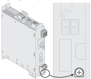
• Connect the ground connection of the device to the central grounding point of the system.
