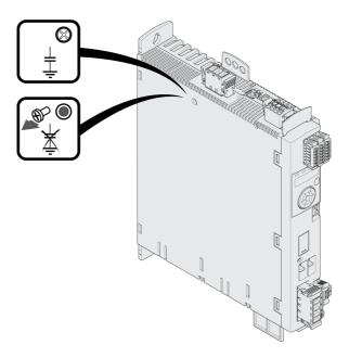
To deactivate the Y capacitors, remove the screw. Keep this screw so you can re-activate the Y capacitors, if required.
