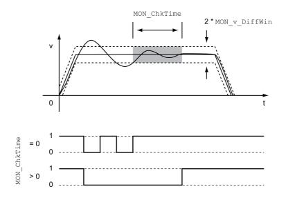
The parameters  ${\tt MON\_v\_DiffWin} \ \ \text{and} \ {\tt MON\_ChkTime} \ \ \text{specify the size of the window}.$
