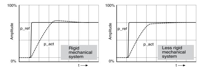
The p gain setting  $CTRL1\_KPp$  ( $CTRL2\_KPp$ ) is optimal if the reference value is reached rapidly and with little or no overshooting.
