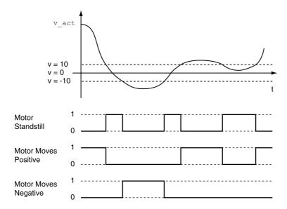
The status is available via signal outputs. In order to read the status, you must first parameterize the signal output functions "Motor Standstill", "Motor Moves Positive" or "Motor Moves Negative", see chapter Digital Inputs and Outputs (see page 196).
