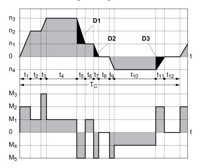
These two characteristics are also used for the rating the motor. The segments of the characteristic curves to be considered are designated by  $D_i$  ( $D_1$  ...  $D_3$ ).
