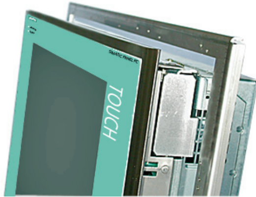
Figure 4-2 Clamping frame with seal
