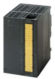
SIPLUS S7-300 SM326F DO8 -25 ... +60 DEGREES C WITH CONFORMAL COATING BASED ON 6ES7326-2BF41-0AB0. DIGITAL OUTPUT F-DO 8 X DC 24V/2A PM FAILSAFE DIGITAL OUTPUT P-M SWITCHING UP TO CATEGORY 4 (EN954-1), SIL 3 (IEC 61508)
