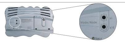
The Power Panel 65 device is equipped with 2 hex switches that can be used as operating mode or node number switches. Switch positions 0x01 to 0xFE are used to set the INA station number of the Ethernet interface.
