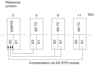
Figure 5-2 Example of assigning parameters of reference junctions
