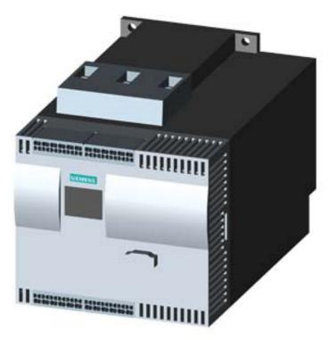
SIRIUS soft starter Values at 400 V, 40  $^{\circ}$ C Standard: 47 A, 22 kW Inside-delta: 81 A, 45 kW 200-460 V AC, 230 V AC spring-type terminals
