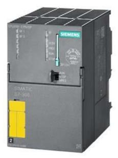
\*\*\* SPARE PART\*\*\* SIMATIC S7-300 CPU315F-2 PN/DP, CENTRAL PROCESSING UNIT WITH 256 KBYTE WORKING MEMORY, 1. INTERFACE MPI/DP 12MBIT/S, 2. INTERFACE ETHERNET PROFINET, MICRO MEMORY CARD NECESSARY USEABLE WITH SOFTWARE OPTION S7 DISTRIBUTED SAFETY V5.4 OR HIGHER
