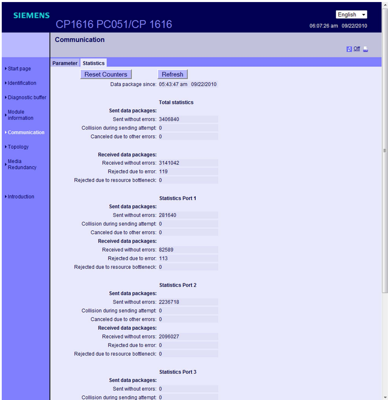
Figure 4-13 Characteristic data of data transfer
