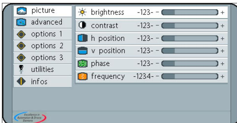
The OSD varies depending from the represented signal-source. OSD functionality by represented RGB (VGA)-signal and DVI signal are described in the following captures.
