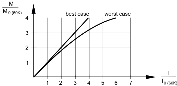
Figure 4-4 Torque-current characteristic curve for self-cooled motors
