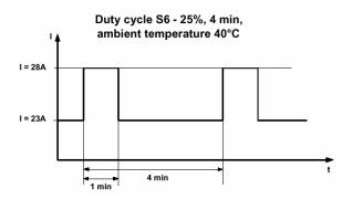
25A at 40°C ambient temperature 28A at 40°C ambient temperature
