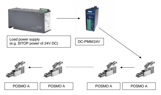
The DC-PMM/24V is connected directly after the load power supply and before the first POSMO A, with terminals L+ Input and M (existing three times altogether) of the PMM to be wired to the load power supply, terminals L+ Output and M to be wired to the first motor.
