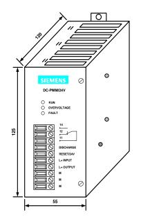
Abmessungen / Dimensions: 125 mm x 120 mm x 55 mm
