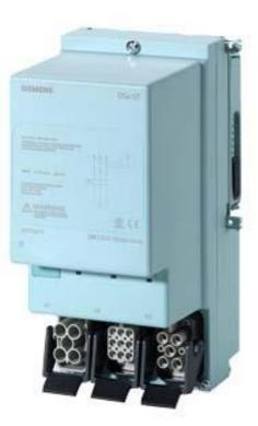
ET 200PRO DSE ST DIRECT STARTER STANDARD; MECH. SWITCHING; ELECTRO. UE PROTECTION; 3PH 400 V/0.9KW; 0.15A...2.00A BRAKE CONTACT AC 400V; HAN Q4/2 - HAN Q8/0
