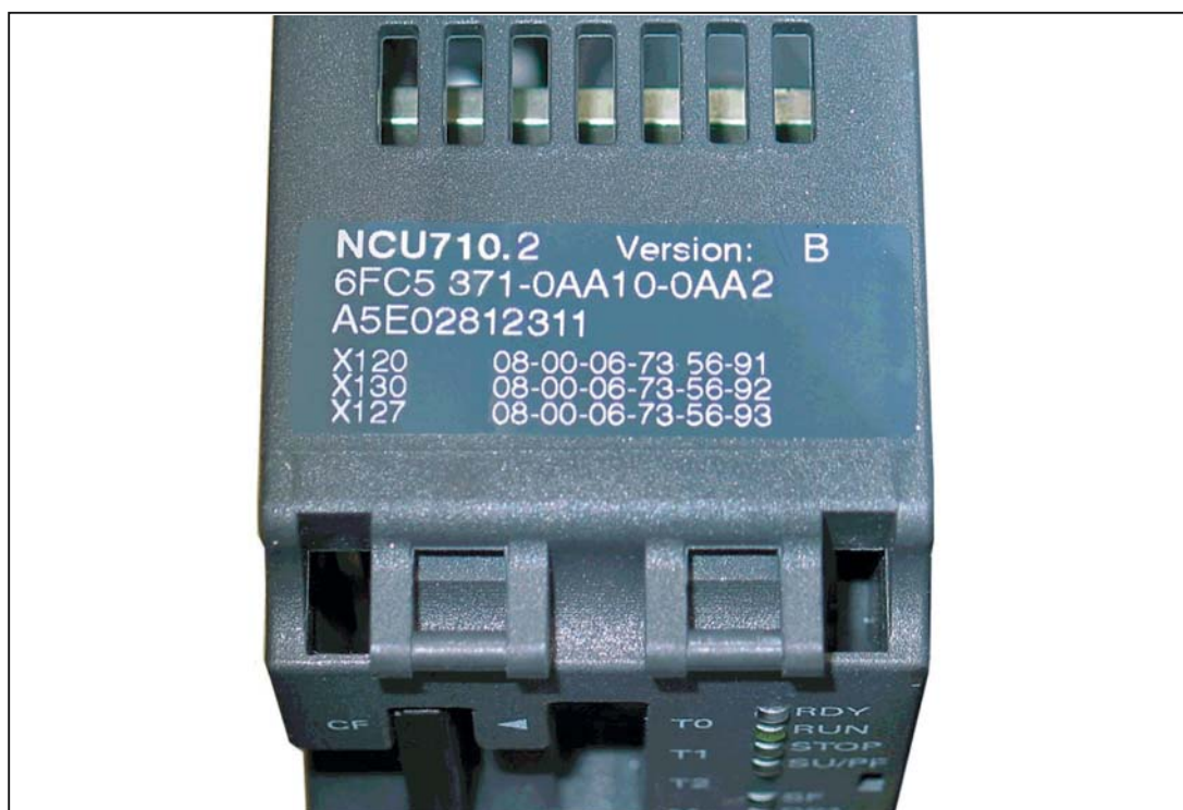
Figure 7-6 MAC addresses of Ethernet interfaces X120, X130, X127
