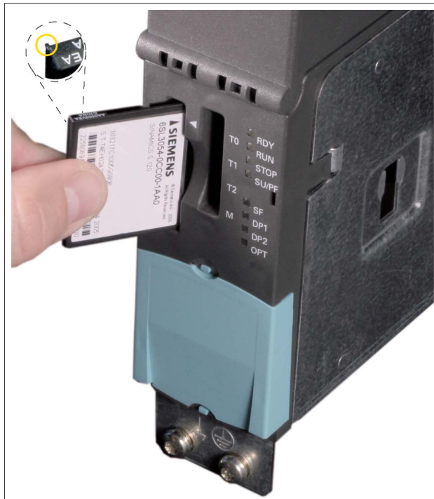
Figure 10-3 Inserting the CompactFlash card
