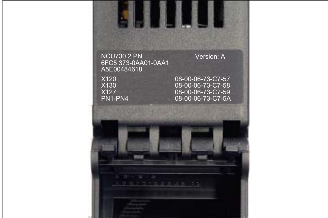
Figure 7-8 MAC addresses of the PROFINET/Ethernet interfaces
