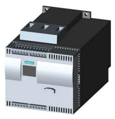
SIRIUS soft starter Values at 400 V, 40 °C Standard: 57 A, 30 kW Inside-delta: 99 A, 55 kW 200-460 V AC, 230 V AC Screw terminals
