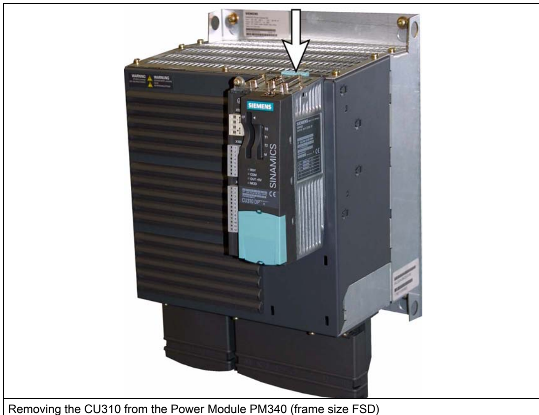
Removing the CU310 from the Power Module PM340 (frame size FSD)
