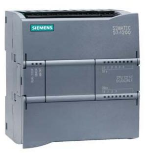
\*\*\* SPARE PART\*\*\* SIMATIC S7-1200, CPU 1211C, COMPACT CPU, DC/DC/RELAY, ONBOARD I/O: 6 DI 24V DC; 4 DO RELAY 2A; 2 AI 0 - 10V DC, POWER SUPPLY: AC 20.4 - 28.8 V DC, PROGRAM/DATA MEMORY: 25 KB
