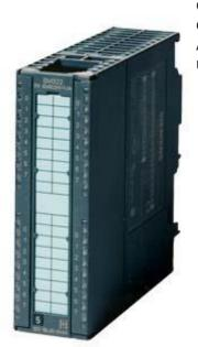
SIPLUS S7-300 SM322 - 40-POLE -25 ... +60 DGR C WITH CONFORMAL COATING CONFORMITY WITH EN50155 T1 CAT 1 CL A/B BASED ON 6ES7322-1HF10-0AA0 . DIGITAL OUTPUT OPTIC. ISOLATED 8 DO (RELAY), 1 X 40-POLE, 24V DC, 5A OR AC 230V, 5A, CONNECT. WITH SPRING TERMINALS CAN BE USED WITH 6ES7392-1BM01-0AA0 AN HIGHER
