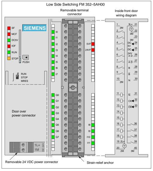
Figure 4-1 Front Terminal Connector of the FM 352-5AH00 (Low Side Outputs)
