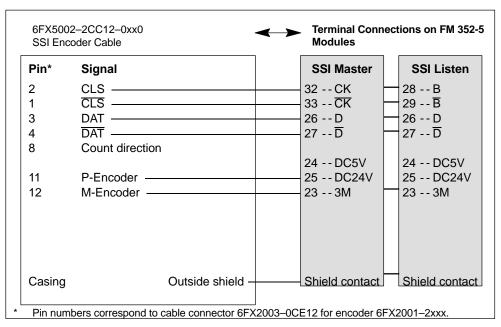
Figure 4-5 Wire Connections for SSI Encoder from SSI Encoder Cable
