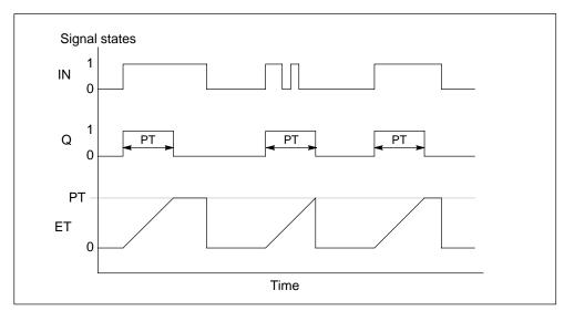
Figure 6-43 Timing Diagram for Pulse Timer (TP)
