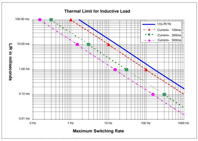
Figure A-8 Graph 2 Thermal for Inductive Load
