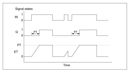
Figure 6-44 Timing Diagram for On-Delay Timer (TON)
