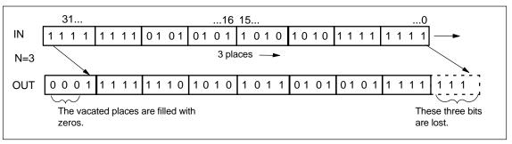
Figure 6-36 Example of Bit Shifts for the SHL\_DW Shift Right Double Word Instruction
