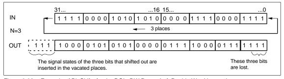
Figure 6-38 Example of Bit Shifts for the ROL\_DW Rotate Left Double Word Instruction
