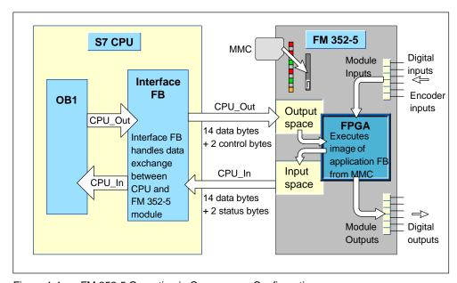
Figure 1-1 FM 352-5 Operation in Coprocessor Configuration
