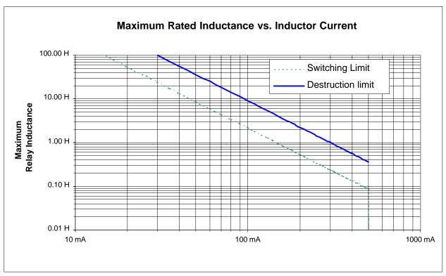
Figure A-7 Graph 1 Maximum Rated Inductance vs. Inductor Current
