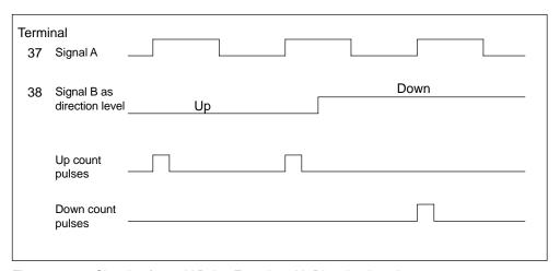
Figure 7-5 Signals of a 24 V Pulse Encoder with Direction Level
