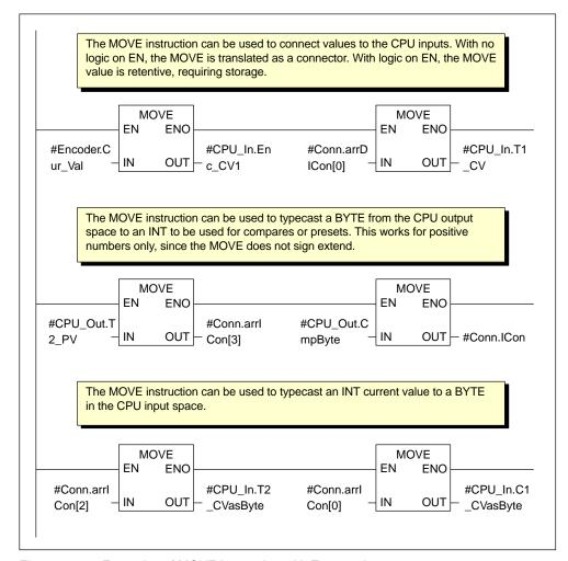
Figure 6-10 Examples of MOVE Instruction with Typecasting
