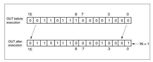
Figure 6-54 Example of BitShift\_W and BitShift\_DW
