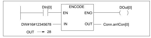
Figure 6-48 Example of the Encode Binary Position Function
