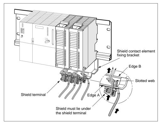
Figure 4-6 Attaching Shielded Cables to Shield Contact Element
