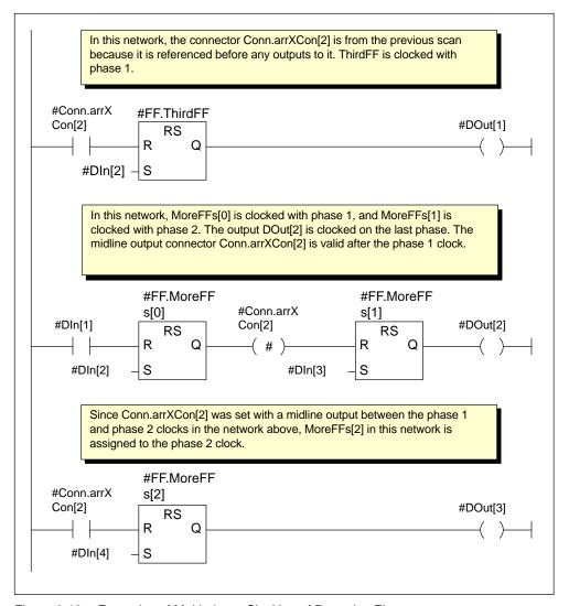
Figure 6-13 Examples of Multi-phase Clocking of Retentive Elements
