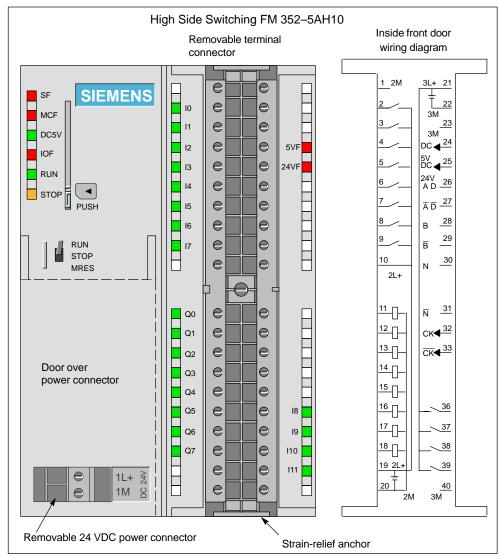
Figure 4-2 Front Terminal Connector of the FM 352-5AH10 (High Side Outputs)
