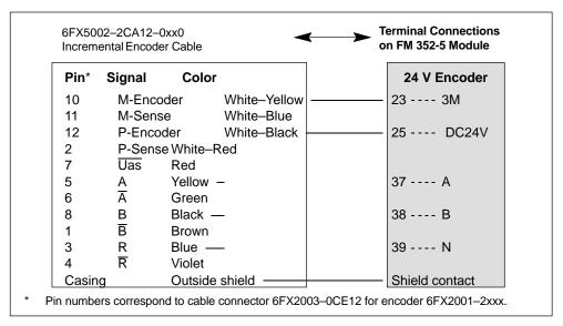
Figure 4-4 Wire Connections for 24 V Encoder from Incremental Encoder Cable
