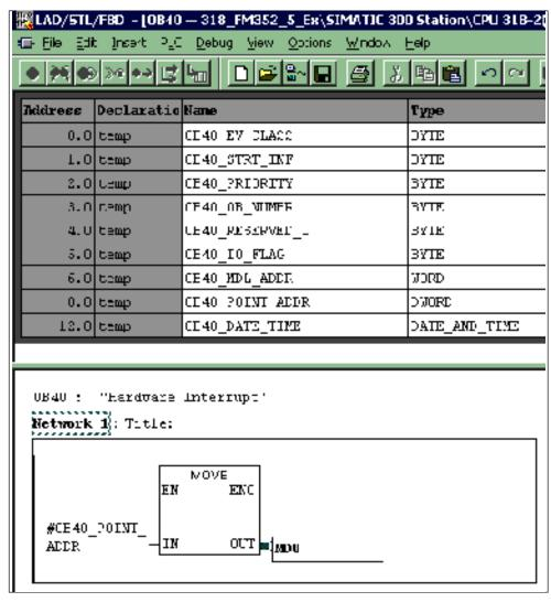
Figure 8-1 Accessing the OB40 Interrupts through Ladder Logic
