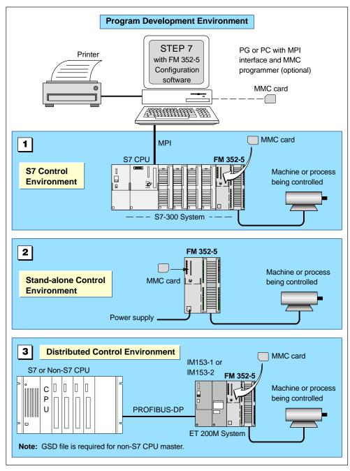
Figure 1-3 Examples of System Configurations
