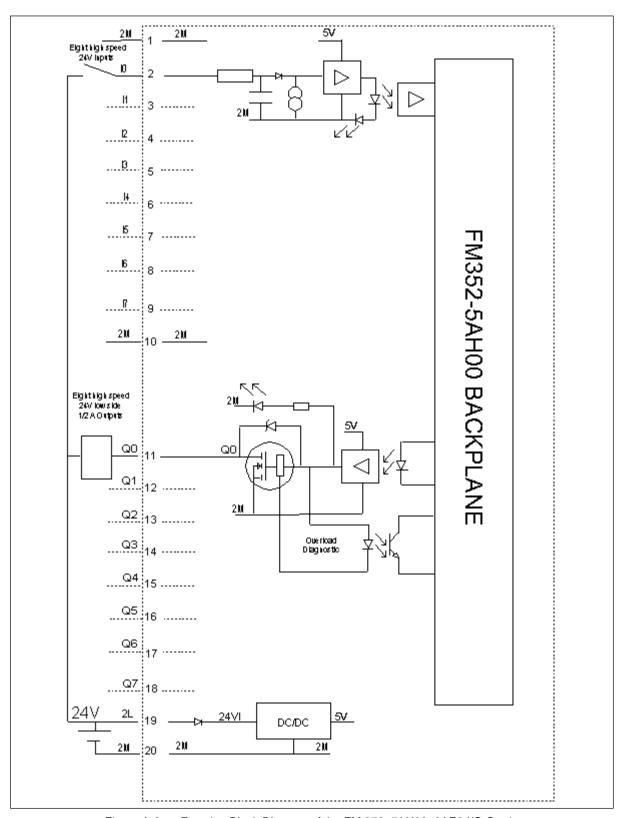
Figure A-3 Function Block Diagram of the FM 352–5AH00–0AE0 I/O Card
