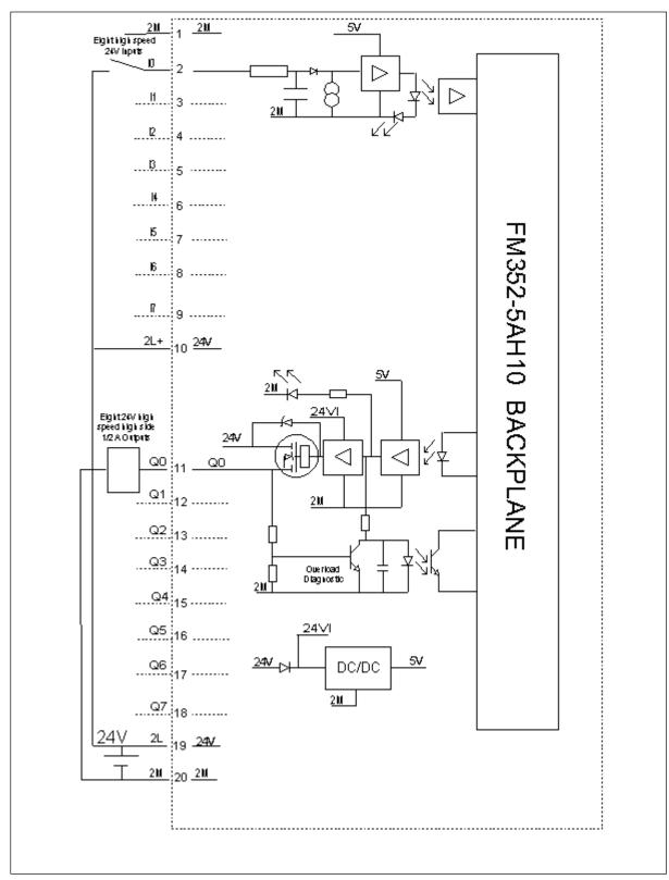
Figure A-2 Function Block Diagram of the FM 352–5AH10–0AE0 I/O Card
