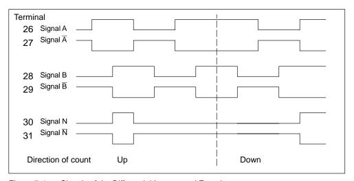
Figure 7-4 Signals of the Differential Incremental Encoder
