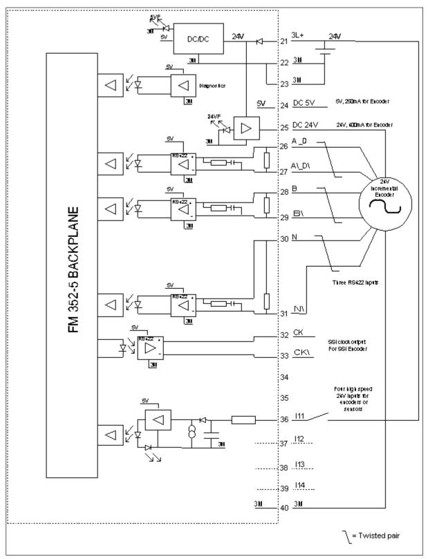
Figure A-4 Function Block Diagram of the FM352–5AHx0 Encoder Card
