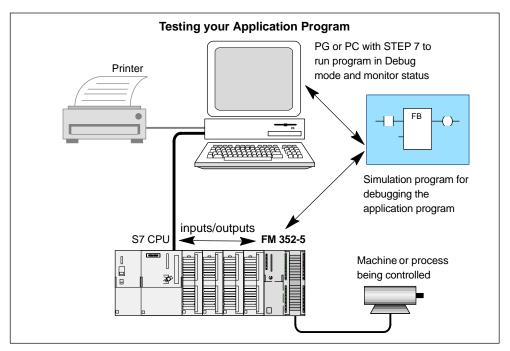
Figure 1-4 System Configuration for Debugging your Program
