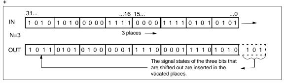
Figure 6-40 Example of Bit Shifts for the ROR\_DW Rotate Right Double Word Instruction
