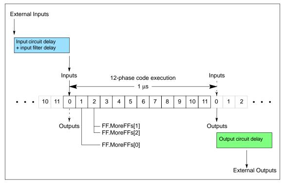
Figure 6-14 Multi-Phase Clocking and I/O Timeline
