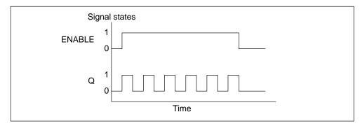
Figure 6-46 Timing Diagram for Clock Pulse Generator (CP\_Gen)
