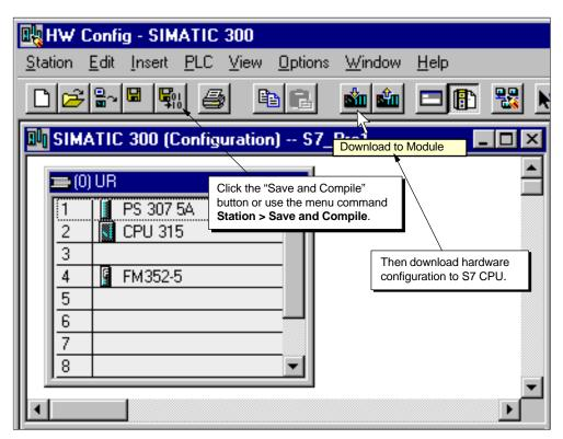
Figure 5-7 Saving and Compiling the Hardware Configuration
