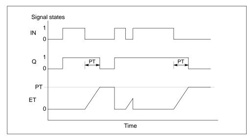
Figure 6-45 Timing Diagram for Off-Delay Timer (TOF)
