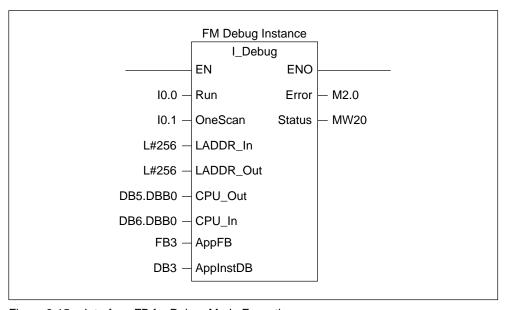
Figure 6-15 Interface FB for Debug Mode Execution
