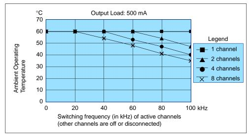
Figure A-5 Switching Frequency vs. Ambient Temperature at 500 mA Output Load
