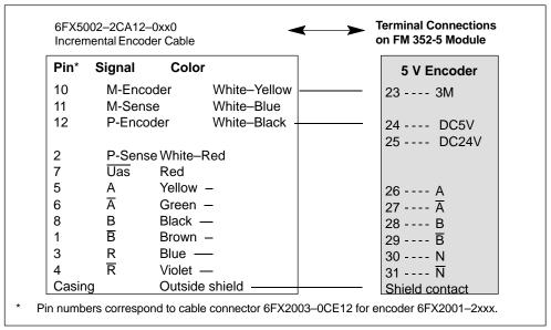
Figure 4-3 Wire Connections for 5 V Encoder from Incremental Encoder Cable
