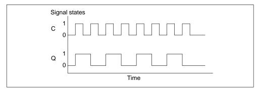
Figure 6-42 Timing Diagram for Binary Scaler (BiScale)
