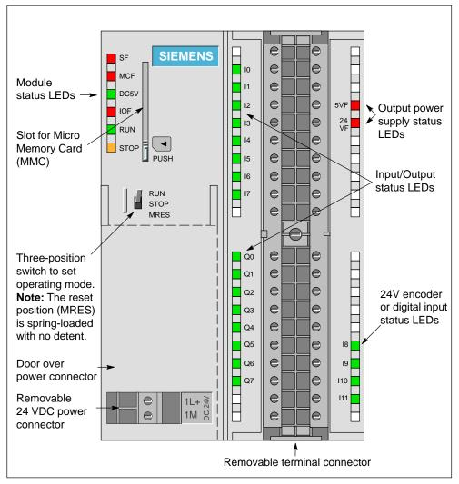
Figure 1-2 Main Features of the FM 352-5 Module
