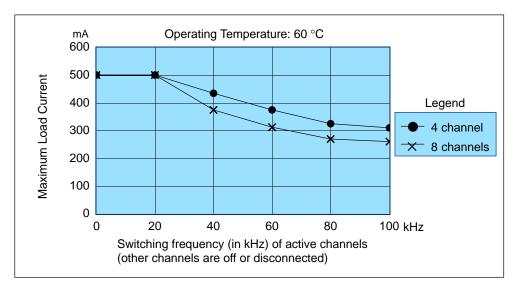
Figure A-6 Switching Frequency vs. Maximum Output Current at 60 °C
