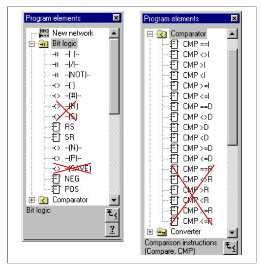
Figure 6-2 Valid Bit Logic and Comparator Instructions from STEP 7 for the FM 352-5
