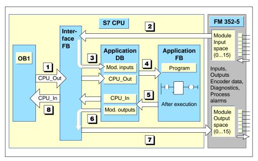
Figure 6-16 Data Exchange in Debug Mode
