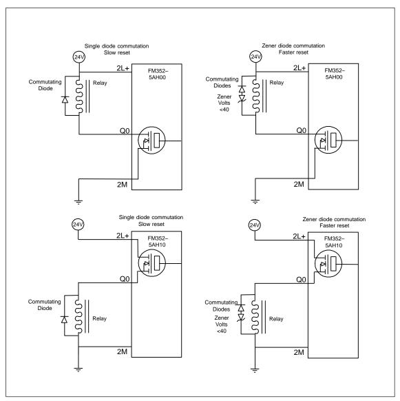
Figure A-9 Application of Commutation Diodes
