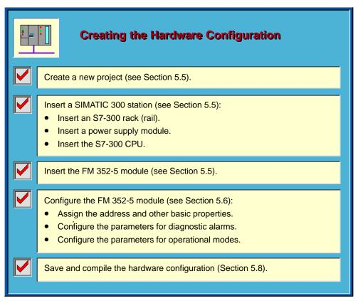
Figure 5-2 Installing and Configuring the Hardware
