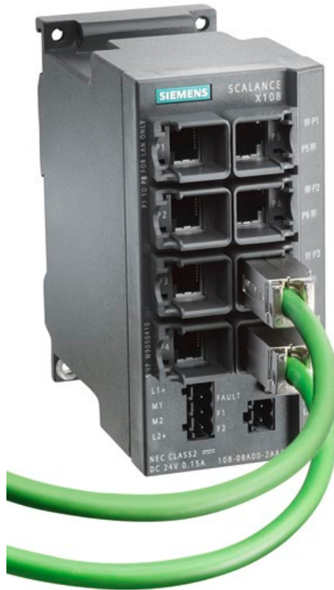
Figure 5-2 Plugging in the IE FC RJ45 Plug 180
