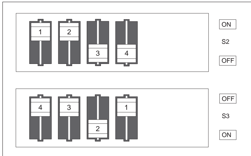
Figure 2-1 Standard Setting of the Switches S2 (1 to 4) and S3 (1 to 4) for 266 MHz Pentium PII CPU
