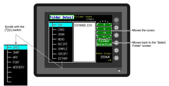
Select the desired folder using the [↑]/[↓] switch, and press the [OK] switch.
