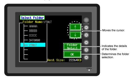
To see the details of the folder, press the [Folder Detail] switch.
