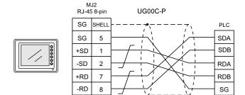
\* When connecting to a Mitsubishi QnA CPU port, a connection between MJ2 and the PLC can be established by changing the PLC-side connecting method.
