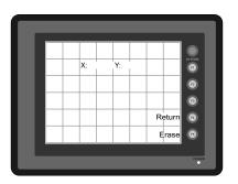
Press a position on the panel, and check that the pressed position turns white.
