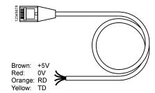
When using the barcode reader that was connected to UG400 (POD's old version), connect it to the D-sub 9-pin female connector using the UG00C-B cable as shown below.
