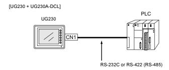
The host link unit of the PLC or the CPU port is used and the UG230 (master station) establishes
