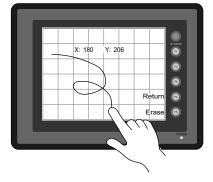
3. If a position different from the pressed position turns white, refer to "Touch Switch Adjustment" on the next page and adjust the touch switch position.
