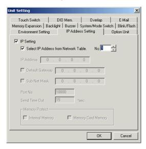
4. Click the [OK] button and transfer the screen data. The IP address set above can be checked on the "Ethernet Information" screen to be displayed from the Main Menu screen.
