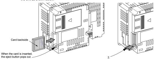
2. To remove the card, press the eject button. The card pops out.
