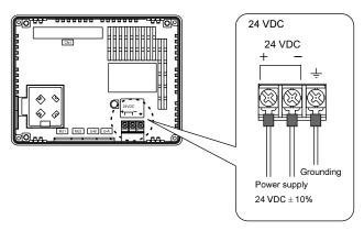
• Tighten terminal screws on the power supply terminal block with the following torque.
