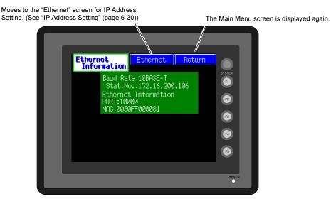
Pressing the [Ethernet] switch brings up the "Ethernet" screen for IP address setting.
