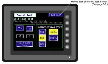
This is a signal test for communications through the MJ1, MJ2 or CN1 connector. Perform this test if the communication is not successful when transferring screen data through MJ1. connecting the PLC using MJ2 or CN1, or selecting multi-link 2, temperature controller/PLC2Way or PLC for MJ1, or connecting the card recorder or serial extension I/O.
