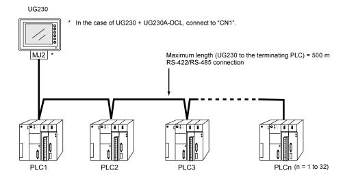
For more information on wiring and communication settings, refer to the User's Manual <PLC Connection> (FEH380).
