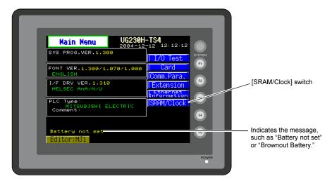
When the [SRAM/Clock] switch on the Main Menu screen is pressed, the following "SRAM/Clock Adjustment" screen appears.
