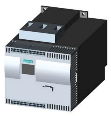
SIRIUS soft starter Values at 400 V, 40 °C Standard: 36 A, 18.5 kW Inside-delta: 62 A, 30 kW 200-460 V AC, 230 V AC spring-type terminals
