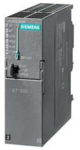
SIPLUS S7-300 CPU 315-2DP -25 ... +70 DEGREES C WITH CONFORMAL COATING BASED ON 6ES7315-2AH14-0AB0 . CPU WITH MPI INTERFACE INTEGRATED 24 V DC POWER SUPPLY 256 KBYTE WORKING MEMORY 2. INTERFACE DP-MASTER/SLAVE MICRO MEMORY CARD NECESSARY
