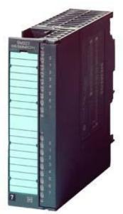
SIPLUS S7-300 SM323 - 20-POLE -40 ... +70 DGR C WITH CONFORMAL COATING CONFORMITY TO EN50155 T1 CAT 1 CL A/B BASED ON 6ES7323-1BH01-0AA0 . DIGITAL MODULE OPTICALLY ISOLAT 8 DI AND 8 DO, 24V DC, 0.5A AGGREGATE CURRENT 2A
