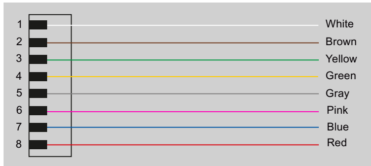
Figure 5-9 Wiring diagram M8 connector
