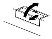
(2) Insert the CF Card in the CF Card Slot, until the eject button is pushed forward.
