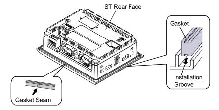
(4) Check that the gasket is attached correctly to the ST.
