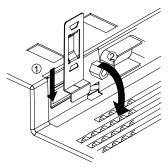
(2) Pass the band of the USB cable clamp through the bridge of the USB holder.
