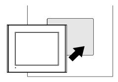
(2) Mount the four panel-mounting brackets on the right and left sides, or the top and bottom sides of the panel to secure the panel.
