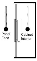
• Be sure that heat from surrounding equipment does not cause the ST to exceed its standard operating temperature.
