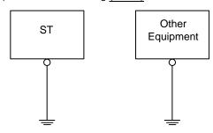
• When supplying power to the ST unit, be sure to separate the input/output and power lines, as shown. [diagram (a)]
