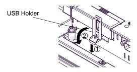
(2) Pass the band of the USB cable clamp through the bridge of the USB holder.
