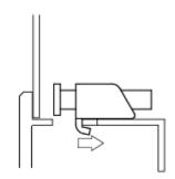
(4) Use a Phillips screwdriver to tighten each fastener screw and secure the ST in place.
