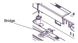
(3) Insert the USB cable into the port. Fasten the band around the plug and secure it with the clamp.
