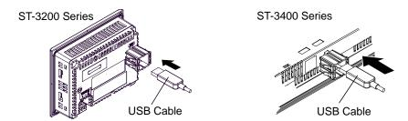
(4) Attach the USB cover to attach the USB cable. Insert the USB cover into the tab of the USB holder.
