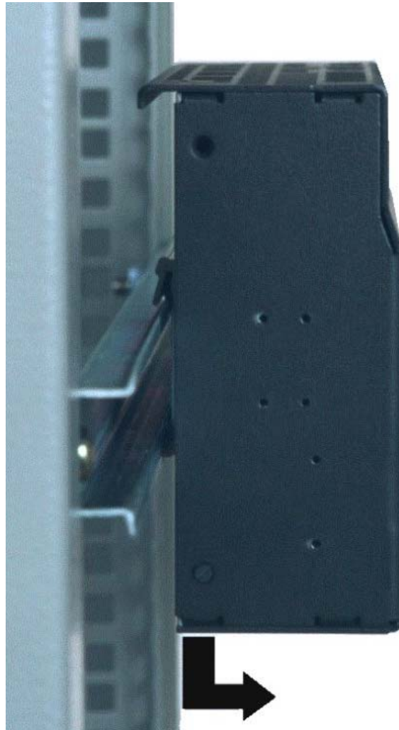
Figure 13. Removing from the Standard Rail
