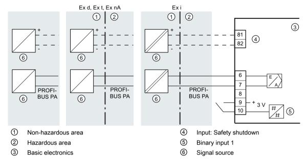
Figure 4-5 Device version with PROFIBUS PA
