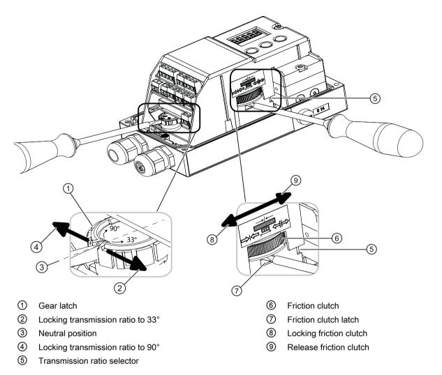
Figure 3-2 Locking friction clutch and transmission ratio
