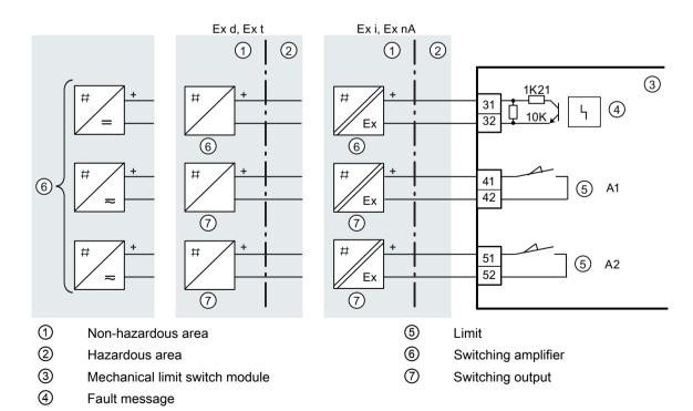
Figure 4-10 Mechanical limit switch module
