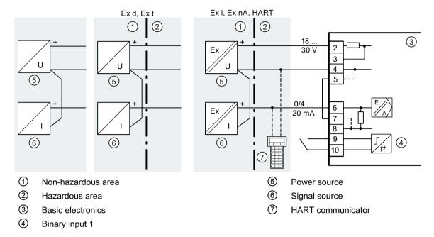
Figure 4-3 Device version 2-/3-/4-wire, with wiring type 3-wire
