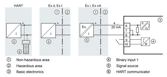
Figure 4-1 Device version 2-wire
