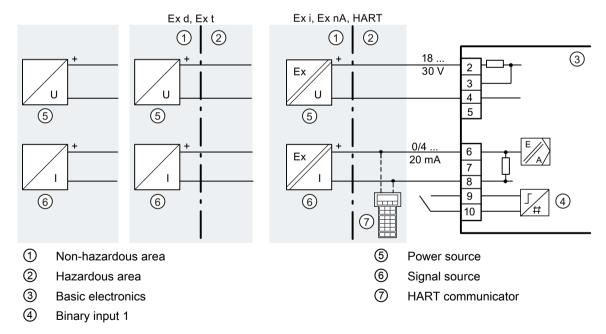
Figure 4-4 Device version 2-/3-/4-wire, with wiring type 4-wire
