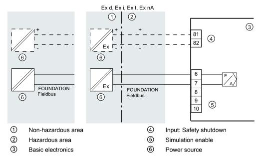
Figure 4-6 Device version with FOUNDATION Fieldbus
