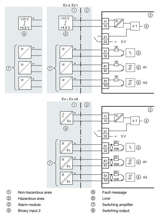
Figure 4-7 Alarm module
