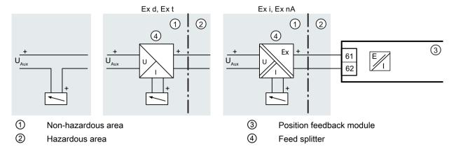
Figure 4-8 Position feedback module
