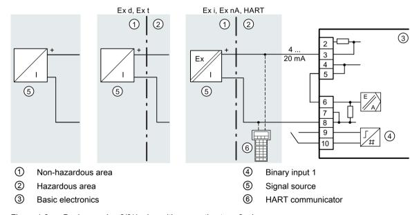
Figure 4-2 Device version 2/3/4-wire, with connection type 2-wire
