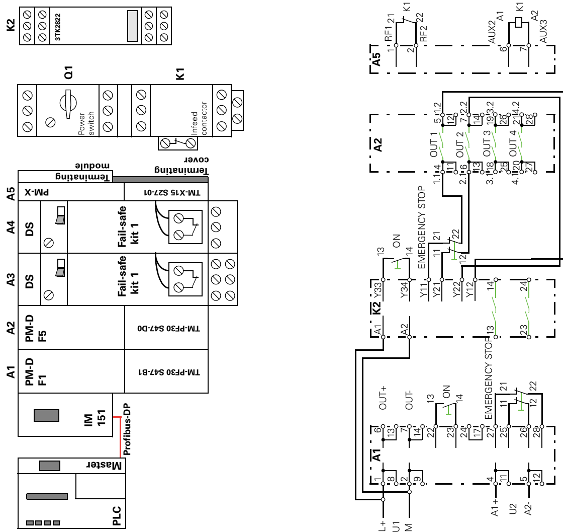
Figure 11-19: Potential-free connection between an ET 200S safety circuit and autonomous safety circuits
