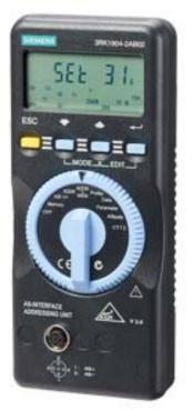
AS-INTERFACE ADDRESSING UNIT V3.0 FOR SETTING ADDRESSES OF AS-I SLAVE MODULES, INPUT/OUTPUT TEST AND OTHER FUNCTIONS. AS-I SPECIFICATION V3.0, M12 CONNECTION SOCKET, WITH ADDRESSING CABLE 1.5 M (M12 CONNECTOR / HOLLOW PLUG). WITH BATTERIES (4 X 1.5 V LR6). ADDRESSING OF APPLICATION MODULES VIA 3RK1 901-1MA00
