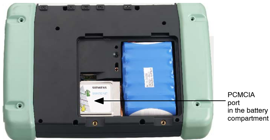
Figure 4-7 Location of the PCMCIA Port in the Battery Compartment
