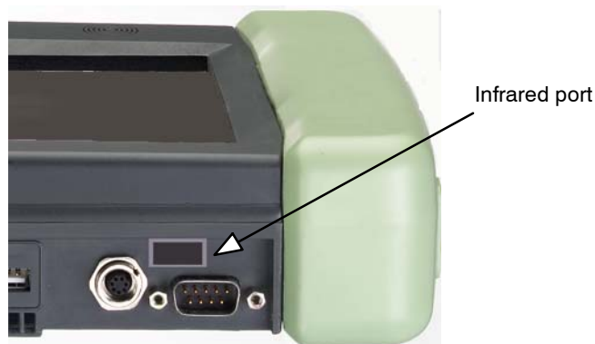
Figure 4-3 Location of the Infrared Port
