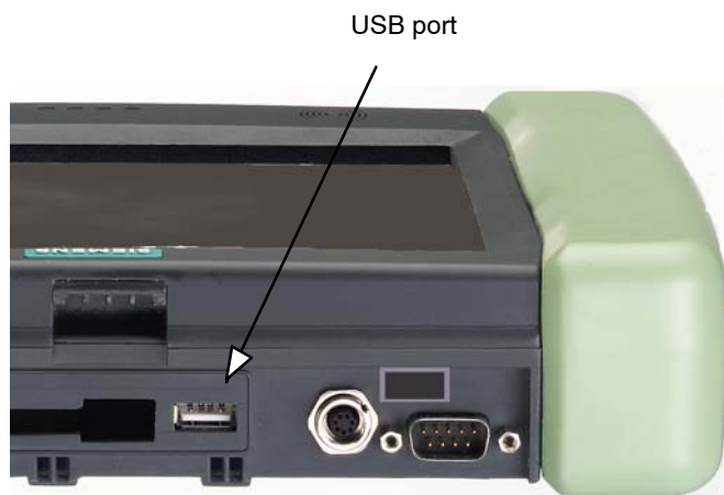
Figure 4-5 Ports under the Protective Cover
