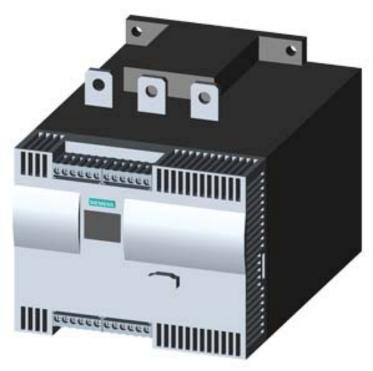
SIRIUS soft starter Values at 460 V, 50  $^{\circ}$ C Standard: 315 A, 250 hp Inside-delta: 546 A, 450 hp 200-460 V AC, 115 V AC Screw terminals
