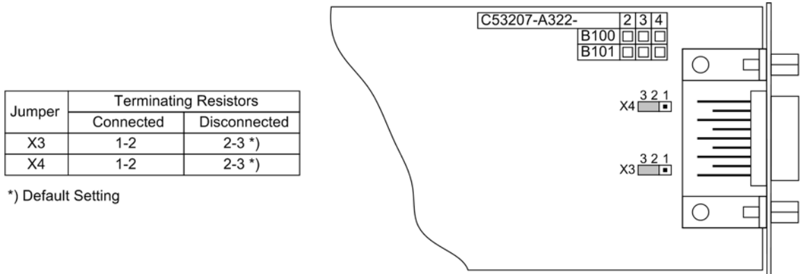
Figure 3-24 Position of the plug-in jumpers for the configuration of the terminating resistors at the Profibus (FMS and DP), DNP 3.0 and Modbus interfaces.
