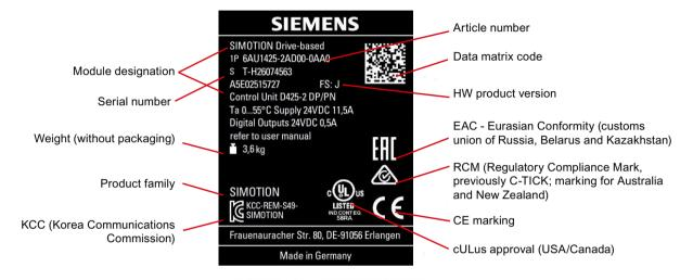
Figure 2-5 Rating plate using the D425-2 DP/PN as an example
