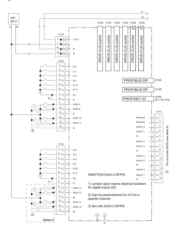
Figure 4-4 Connection and circuit diagram of the digital I/Os
