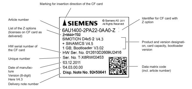
Figure 2-8 Rating plate of the CF card (example of 1 GB CF card)
