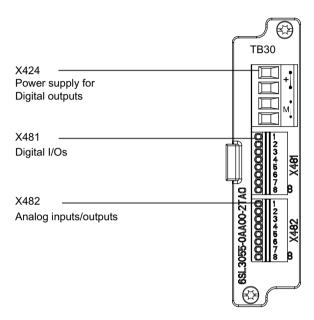
Figure 7-5 Interface arrangement on the TB30
