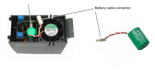
Figure 7-4 Changing the battery in the double fan/battery module
