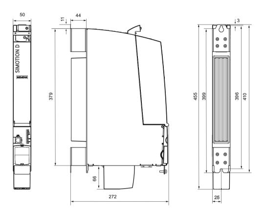
Figure 6-2 D445-2 DP/PN and D455-2 DP/PN dimension drawing
