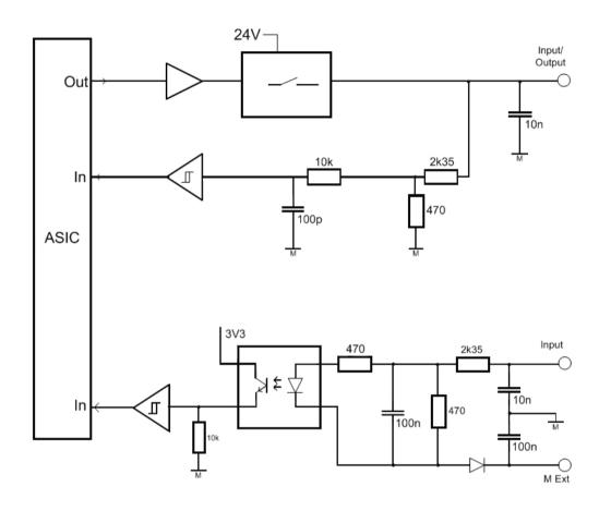
Figure 5-1 SIMOTION D4x5-2/CX32-2 input and output circuits
