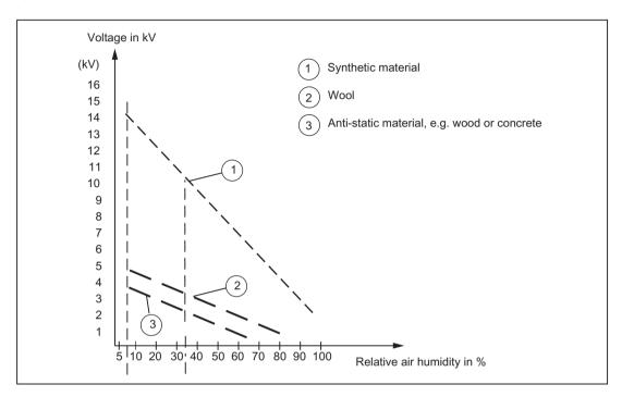
Figure B-1 Electrostatic voltage that can accumulate on operating personnel
