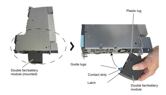
Figure 7-2 Installing the double fan/battery module
