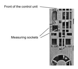
Figure 4-10 Measuring socket position
