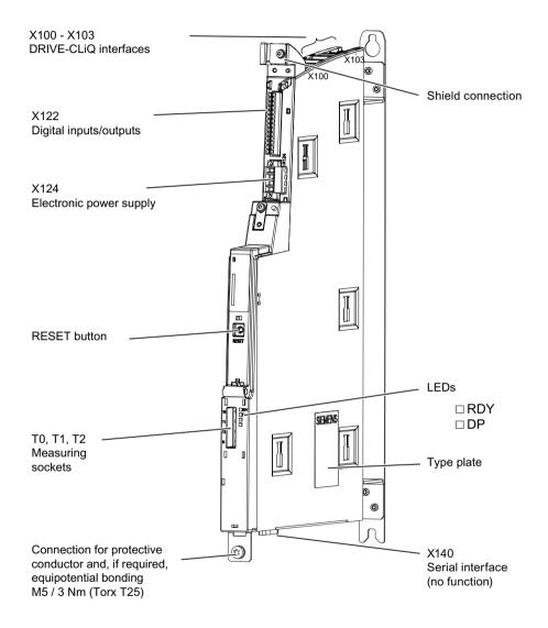
Figure 7-12 CX32-2 (without cover) with interfaces and operator control
