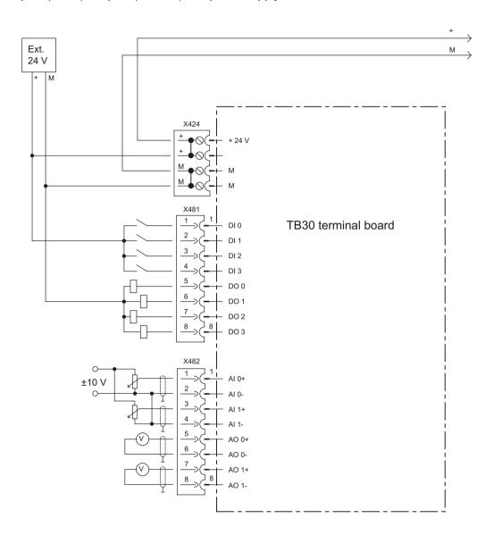
Figure 7-6 TB30 connection diagram
