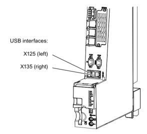
Figure 4-11 The position of the USB X125 and X135 interfaces (example of SIMOTION D4x5-2 DP/PN)
