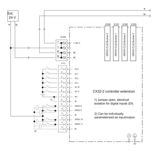
Figure 7-13 Digital I/Os connection diagram
