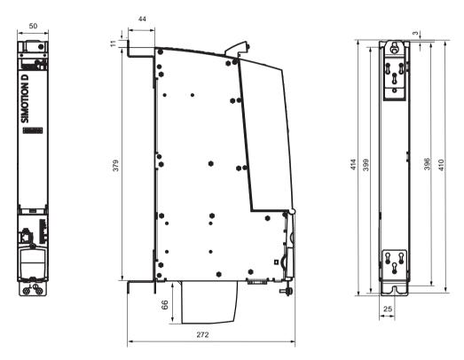
Figure 6-1 D425-2 and D435-2 dimension drawing
