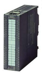
SIMATIC S7/PCS7, SM 321 DIGITAL INPUT MODULE, 16 DI, 24V DC, 1 X 40 PIN, CAPABLE OF DIAGNOSTICS, FOR CONTACTS (CONNECTED/ UNCONNECTED), NAMUR SENSOR, 3/4-WIRE-BERO, WITH FLUTTER MONITORING, PULSE LENGTHENING, WIRE BREAK DETECTION, IM153-2 INTERFACE MOD. REQUIRED
