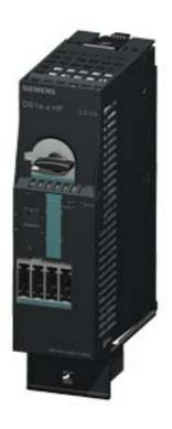
F-DS1E-X FOR ET 200S FAILSAFE DIRECT STARTER SETTING RANGE 0.3...3A MECHANICAL SWITCHING ELECTRONIC PROTECTION EXPANDABLE FOR BRAKE CONTROL MODULE 2DI MODULE SIGNAL FROM CIRCUIT-BREAKER PARAMETERIZABLE
